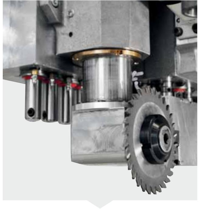
Longitudinal and transversal cuts can be made with the blade unit built into the boring head with 0-90° rotation.
