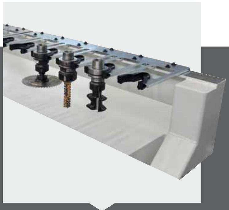
To have the most tools available, the rack magazine may have up to 12 locations, used by all the items present on the machining head.
