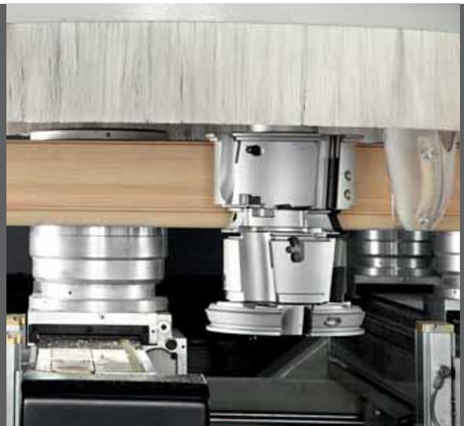
Clean working environment with the conveyor helping to eliminate shavings and sawdust. Available for heads with 3 or 5 axes, it can be used both with single-profile tools and double-profile tools.
