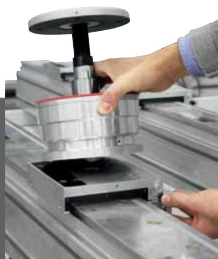
Switching from clamps to suction cups and vice versa is fast and practical. The quick coupling perfected by SCM allows operators to switch at the press of a button, without the need for external tools.
