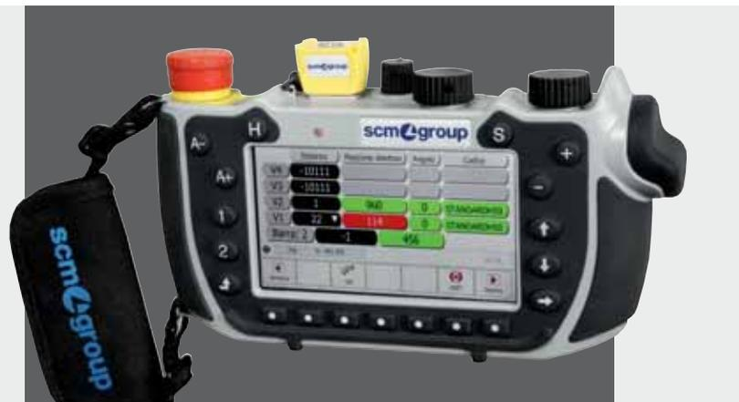
Fast operations that do not require any further checks; the display on the mobile console shows the position for each element and provides a real-time view of all movements until the correct position is reached.
